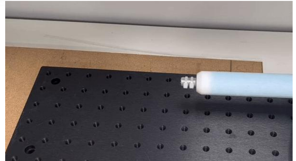
Extension of a SGR with a catheter (KCL, UTH)
