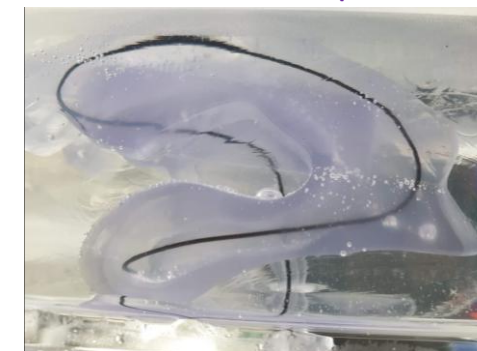
Catheter elongation inside a phantom (KCL)
